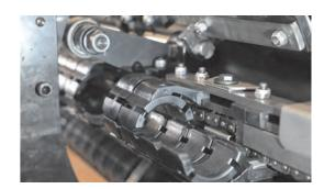
This device is positioned on bearings at the lathe spindle entrance in the area where the loader guides do not support the bar. The device prevents problems of instability and vibration of bars.
